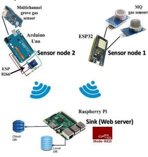
FIG. 1: THE OVERALL SYSTEM HARDWARE COMPONENTS
